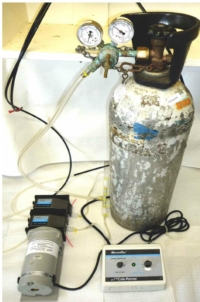
**Fig. 1.** Precise flow of CO<sub>2</sub> is controlled with a pressure regulator and peristaltic pump system. The system shown is running with two pump heads that feed different mesocosms. Size of tubing and pump heads allows simultaneous feeds at two or more levels of acidification.
